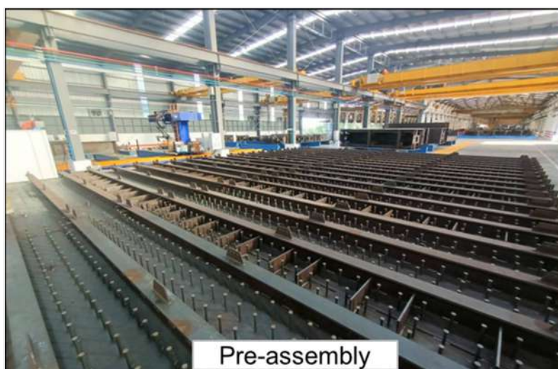
Example image of Mock-up piece for Project 1F Kotaiko 11 Building SC Wall
